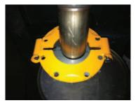
approximate gap of 12-15mm between the 2 clamps. The bolts will be tightened properly later on in the fitting process. Do the same for the second set of clamps at the other end of the catalytic converter.
